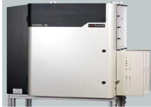
Extrel Max 300IG 2 units (2006/2008) Process MS On-line gas analysis
